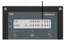
If the temperature alarms are set to ON, a 'T' indication will blink on the display. There are no output changes, but configurations can be made over a network. This is an indication only; ambient temperatures should be measured and the unit calibrated to match. It may take up to 6 hours energised to stabilise temperature readings.
