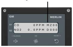
Press [OK] for 5s to activate manual override. Press < > to select the override time (minutes). Press < > to select if the signal relay is included
