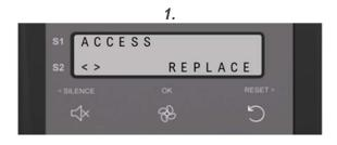
Once the code is accepted use the < and > buttons to access **REPLACE** and press Ok.
