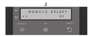
Select the module S1 or S2 using the < > buttons, press OK to confirm.
