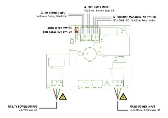
**AC Power Input.** 230V~ supplied to [POWER] connector using a 3-core cable, fused at 3A and the live voltage serves the main isolation switch on the front fascia to cut power to the equipment.
