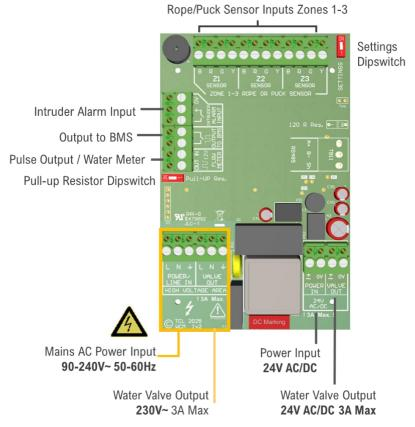
**Note:** Valve voltage and input voltage must match
